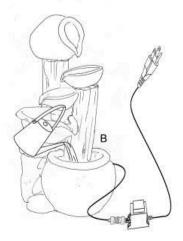
**Step 4:** Finally, connect the plug of pump (C) to a GFCI outlet.
