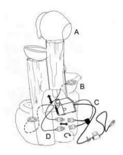
**Step 3:** Fill the basin (B) with clean water, making sure the pump (B) is fully submerged. **Note:** The maximum water level should be approximately 1.2 inches below the top edge of the basin (B).
