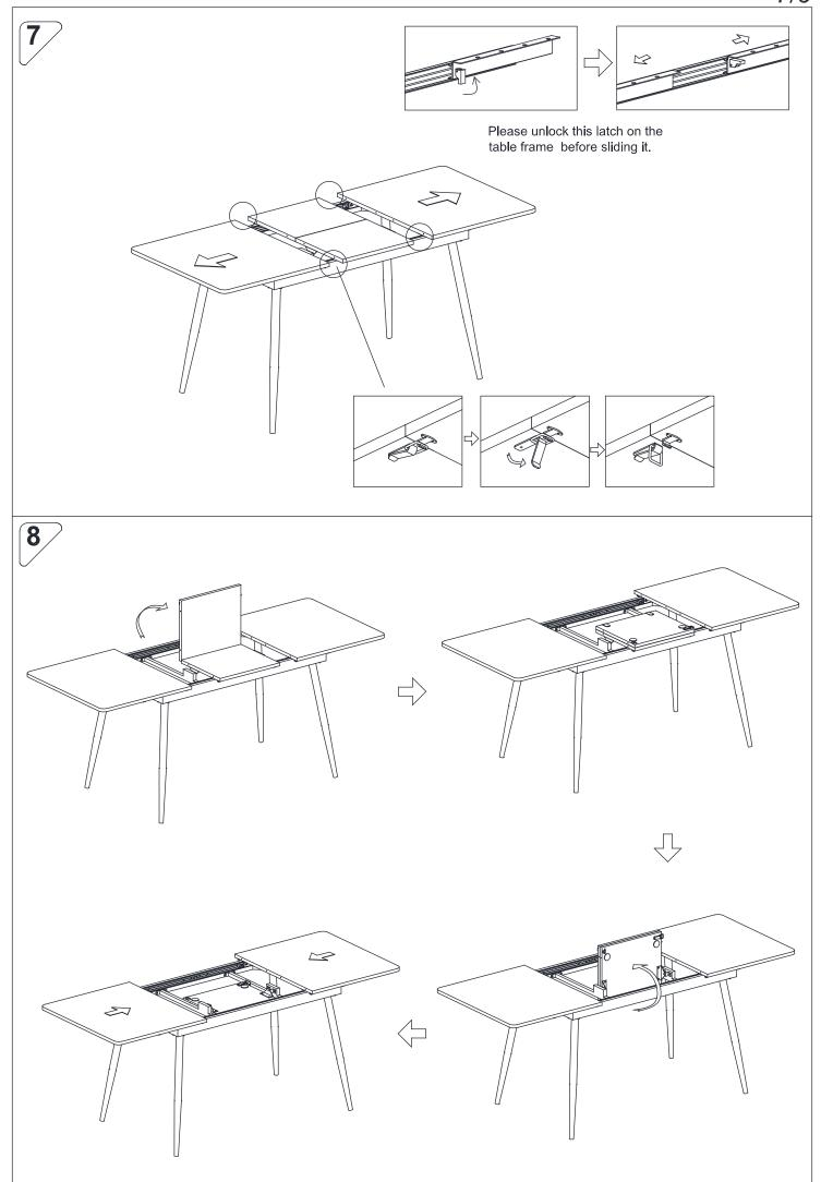
Please lock the latch on the table frame and table board, after shrinking the dining table.
