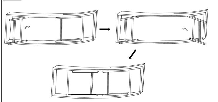
To Close, first colse the leg under the seat, then close the other leg which under back, by hand.
