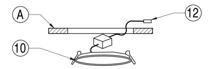
1. First, turn off the power at home. After turning off the power at home, put on insulating gloves to handle it. Connect the wires of the lamp and the wires at home through component #12 (insert several wires into the slot of component #12), and you can use it.
