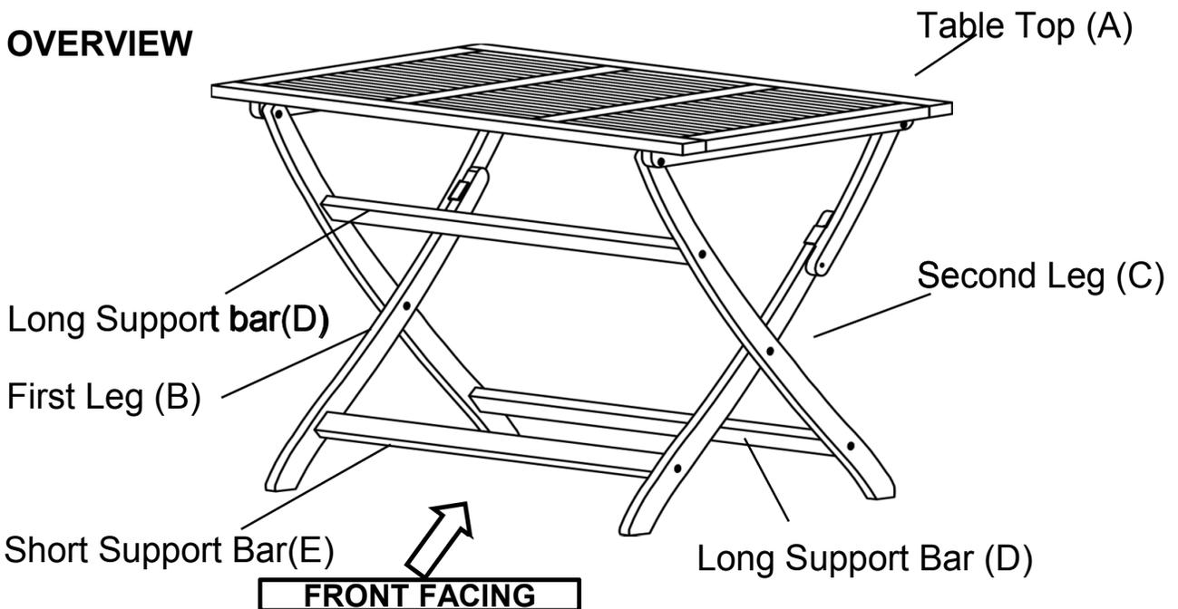
This Table has multiple parts and may require up to 30 minutes to assemble. To give you an overview of the Table parts, the above picture is to help you put the various parts into perspective. Please read through the instruction below to familiarise yourself with the parts and steps before assembly.
