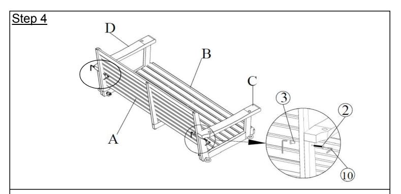
Attach Backrest Panel(A) to Left Arm Panel(C) and Right Arm Panel(D) using Bolts(2) and Sleeve Nuts(3) with Allen Keys(10) as shown above.
