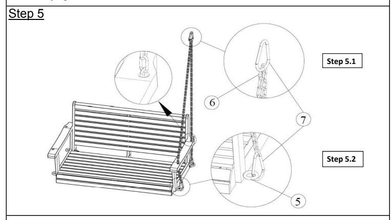
**5.1)** Unscrew the connection on Carabiner( $\bigcirc$ ), then loop the Chain( $\bigcirc$ ) onto the Carabiner( $\bigcirc$ ), and screw the connection shut.
