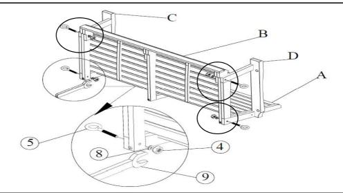
Insert the tenons of the Seat Panel(B) into the mortises of Left Arm Panel(C) and Right Arm Panel(D), then attach using Lock Nuts(4), Washers(8), and Eye Bolts(5), with Wrench(9) as shown above.
