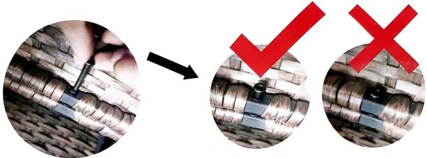
Do not tighten all the bolts in First step.
