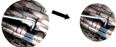
Tighten the bolts by hex wrench until the last step.
