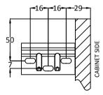
You may need to lengthen the hook's protrusion. To so so, turn screw 'B' anti-clockwise.
