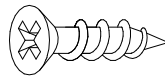
30 x 4 M3.5 x 12mm Screw M3.5 x 12mm de la vis M3.5 x 12mm el tornillo
