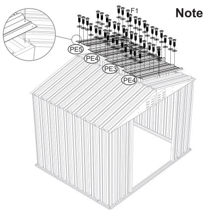
Note: Do not install F1 and V2 in the holes near the outer side of PE5.
