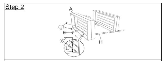
Repeat Step 2 to assemble the Top Shelf (A) using Bolts(①) and the Allen Wrench(⑥).
