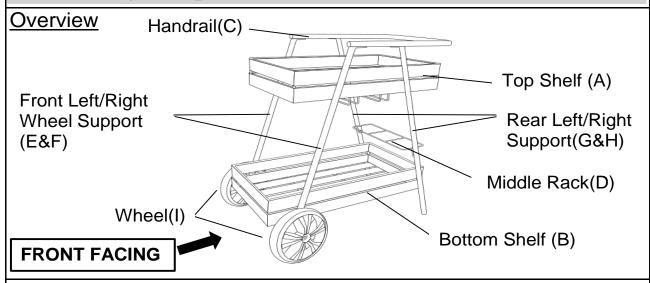
This Bar Cart has multiple parts and may require up to some 30 minutes to assemble. To give you an overview of the Bar Cart parts, the above picture is to help you put the various parts into perspective. Please read through the instructions herebelow to familiarise yourself with the parts and steps before assembly.
