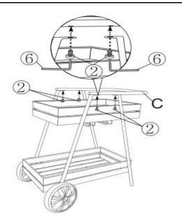
Position the Handrail(C) to the Supports as shown above. Attach the Handrail(C) to the Supports using Bolts(②) and the Allen Wrench(⑤).
