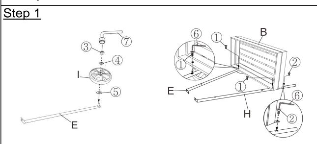
Place the Front Right Wheel Support(E) onto a clean, non-marring surface. Attach the Wheel(I) to the Support(E) using a Washer (4)(5) and Nut(3) with the Allen Wrench(7), tighten the Nut.
