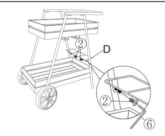
Take out the Middle Rack(D), and attach it using Bolts(②) and the Allen Wrench(⑥).
