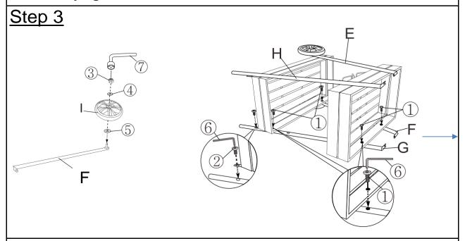
Repeat Step 1 to assemble the Wheel(I) to the Front Left Wheel Support(F). Then, align the Support(F)(G) to the Top and Bottom Shelf(A)(B) as shown above, using  $Bolts(\mathfrak{D})(\mathfrak{D})$  and the Allen  $Wrench(\mathfrak{G})$ .
