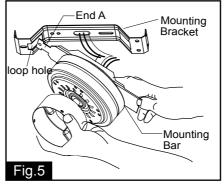
Attach hang motor assembly onto mounting bracket. Insert the End A of mounting bar through the loop hole of the mounting bracket for hands-free wiring.
