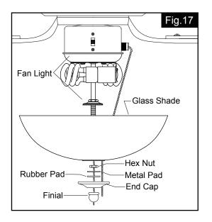
Install the glass shade, rubber washer and metal washer upward through the nipple and secure with hex nut. Then attach the end cap to the glass shade and secure it with finial. Take care to align the holes on the glass shade and the end cap, so the pull chains pass through and move freely.
