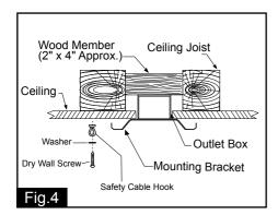
Attach the safety cable hook to the ceiling with the dry wall screw and washer, and make sure the safety cable hook is covered by the fan canopy.
