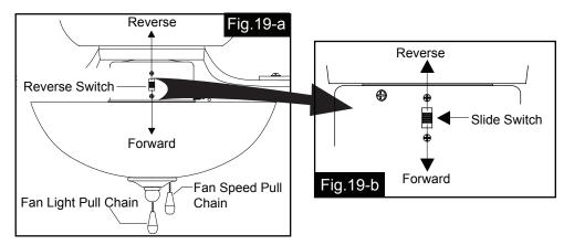
The slide switch sets direction of fan rotation. Select the desired direction of fan rotation. Push the slide switch down for "Forward" and up for "Reverse". CAUTION: If you install a Wall Control for this fan, make sure to use the pull chains to select the "high" position for the fan speed and the "on" position for the fan light.
