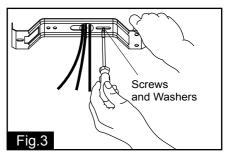
Tighten the mounting bracket to the outlet box with 2 mounting screws and washers. (To reduce the risk of fire, electric shock, or personal injury, mount to the outlet box marked "Acceptable for fan support" and use mounting screws provided with the outlet box.) Pull the electrical wires from the outlet box through the center hole of the mounting bracket for motor wiring installation.
