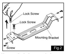
Unscrew the lock screws, lock washers and screws from mounting bracket.
