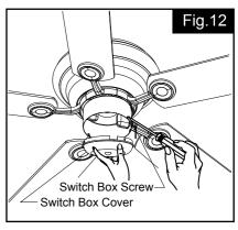
Make sure the wires of the fan light in the switch box are capped with wire nuts. Secure the switch box cover with the switch box screws. To install the fan light, skip this
