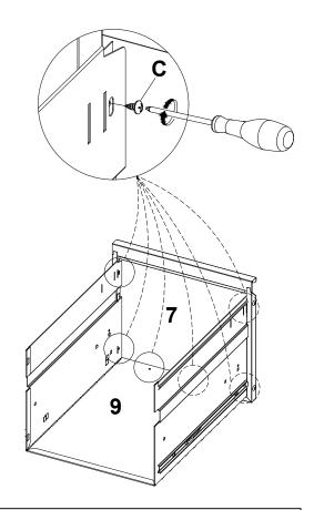
put six screws to hold part 9 into place.
