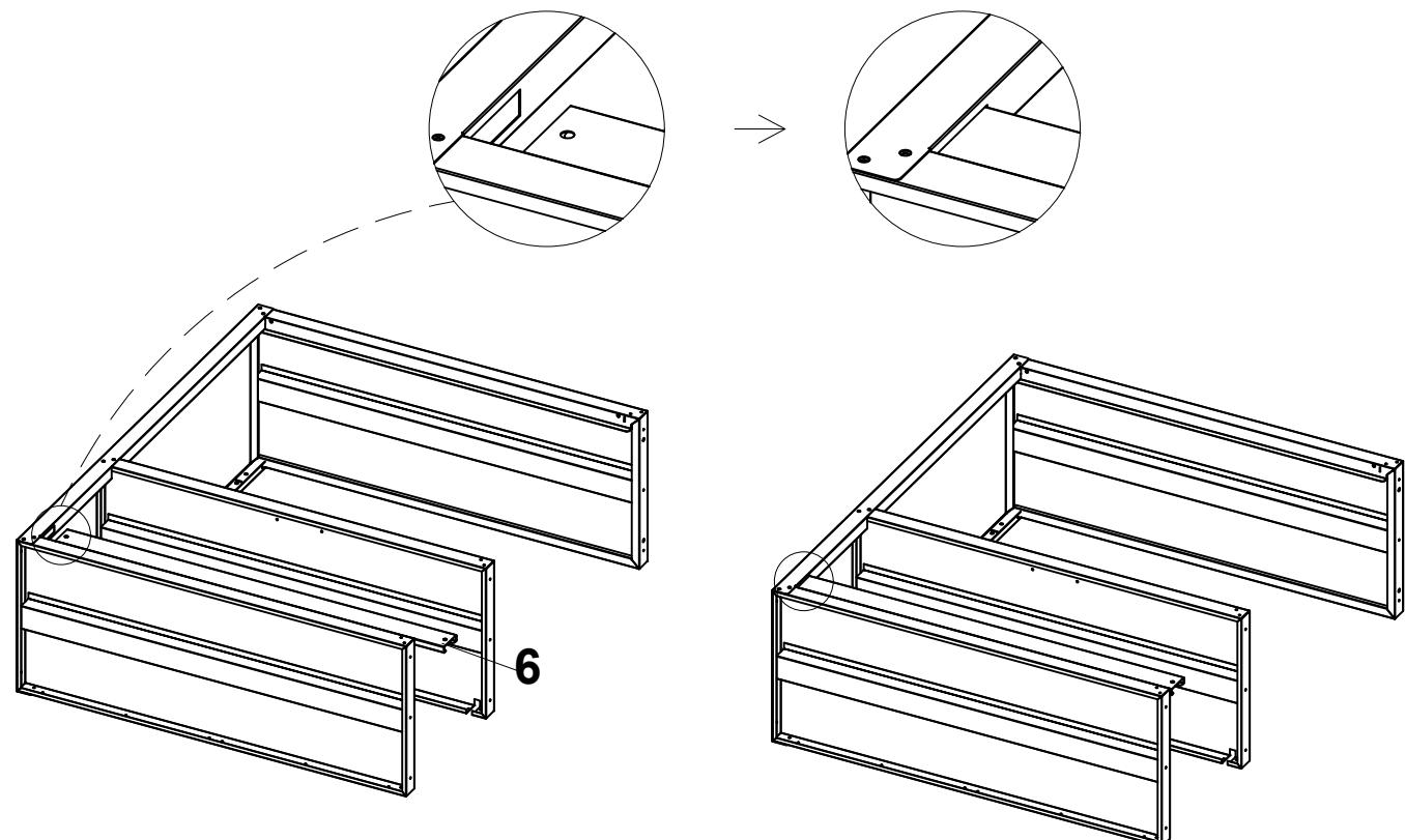
Installation of #6 crossbar Note the direction of installation
