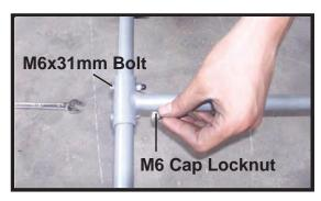
**3** Secure the cross bars to the legs by the M6x31mm Bolts and M6 Cap Locknut.
