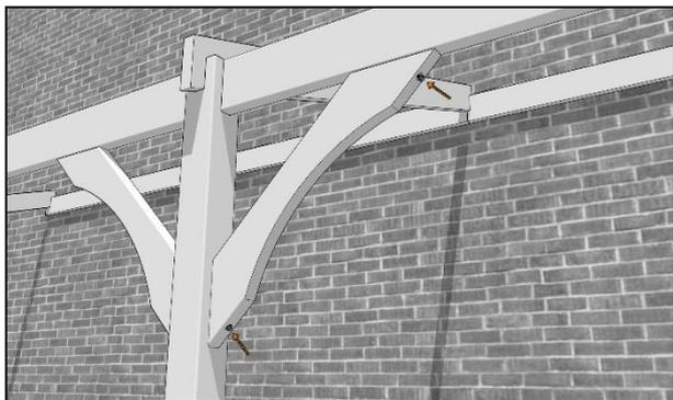
Now fit the final brace into place, Aligning it the underside of the runner and centrally across the inside face of the post. Fix it into place with a 100mm coachscrew at each end.
