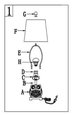
Step 1 Insert the Harp (D) into the Saddle (B). Put the shade(E) on the Harp(D), then tighten the Finial (F)into the Harp (D)
