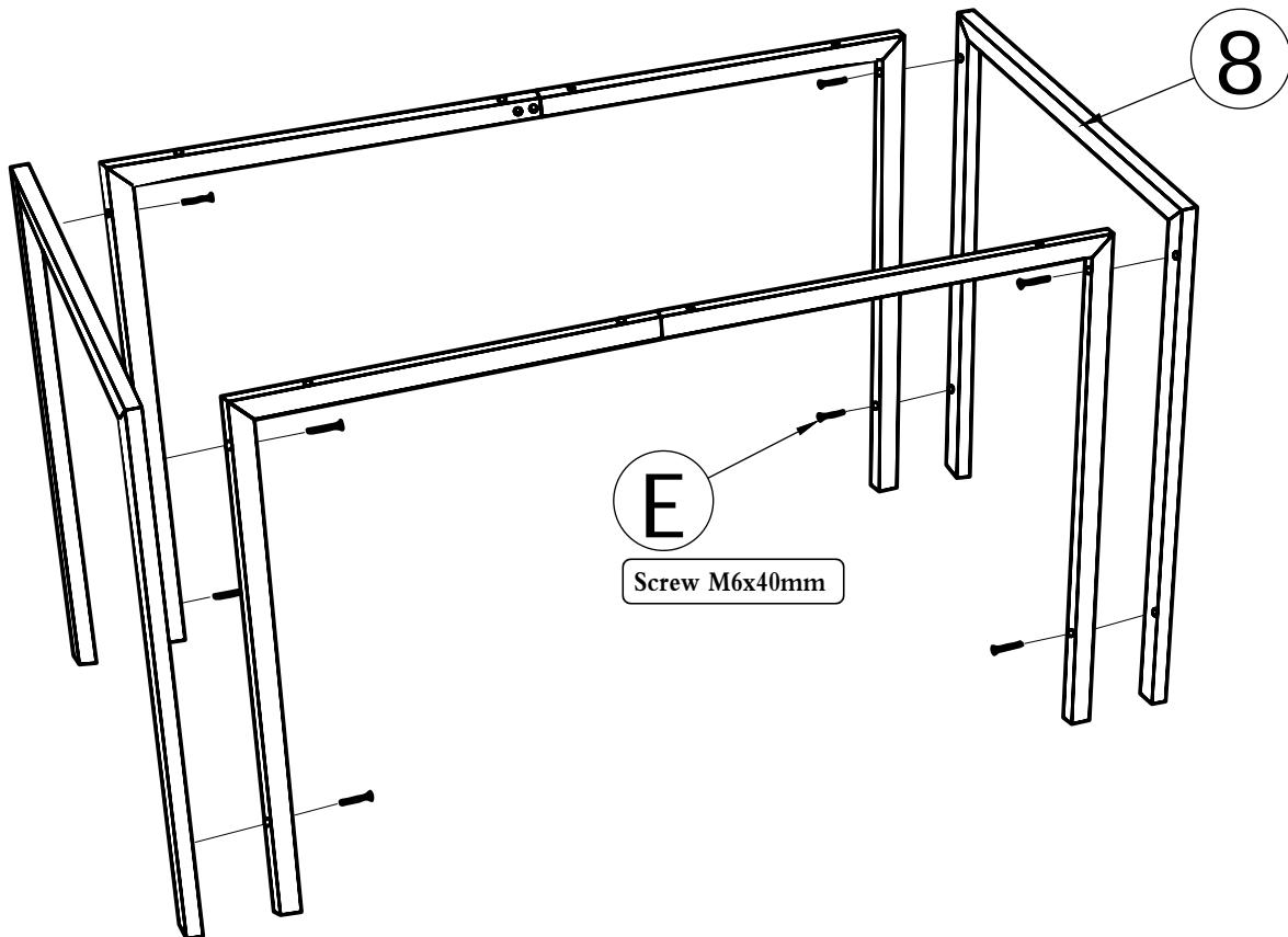
EN-During the assembly, please first half-tighten all the screws into the holes.
