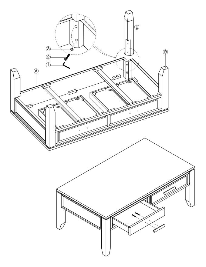
Place the table top (A) up side down on the floor with a piece of cloth or carpet underneath to prevent the finish from scratching. Attach the table leg (B) to the table top corner (A) and secure with lock washer (3) and bolt (2). Tighten bolt (2) with allen key (1). Repeat this step for the remaining three legs.
