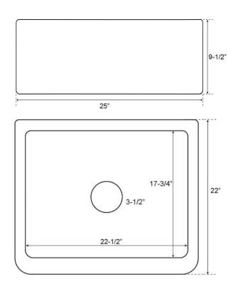
Dimensions of fixture are nominal and may vary within the range of tolerances established by ANSI Standard A112.19.2. Dimensions and specifications subject to change without notice.
