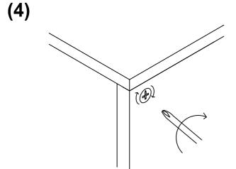
Turn the cam connector with a screwdriver until it will not turn any more with light to moderate force.
