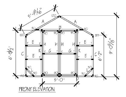
**Step 9:** Finally – measure your structure to determine the amount of materials you will need to purchase to cover your structure. Always make sure you allow for seams or waste material and purchase extra. To determine the amount of material needed for the front and rear of the structure measure the base for your width and then measure from the base to the top of the ridge for your height.
