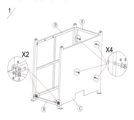
**STEP 1:**Use side panels E to connect and assemble the overall frame.
