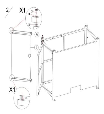
**STEP 2:**Use connecting rods to secure the door to the frame.
