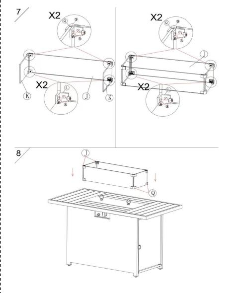
**STEP 7** & 8 :Combine a long glass and a short glass as shown above, and fix the two pieces of glass using glass clasp L and Q, and then use screws to fix the glass clasp. Turn the side of the glass with the gasket down and place the glass cover on the table top.
