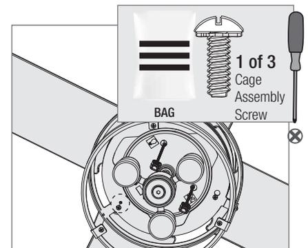
Insert the third cage assembly screw, found in the hardware bag, in place and firmly tighten all the three screws.
