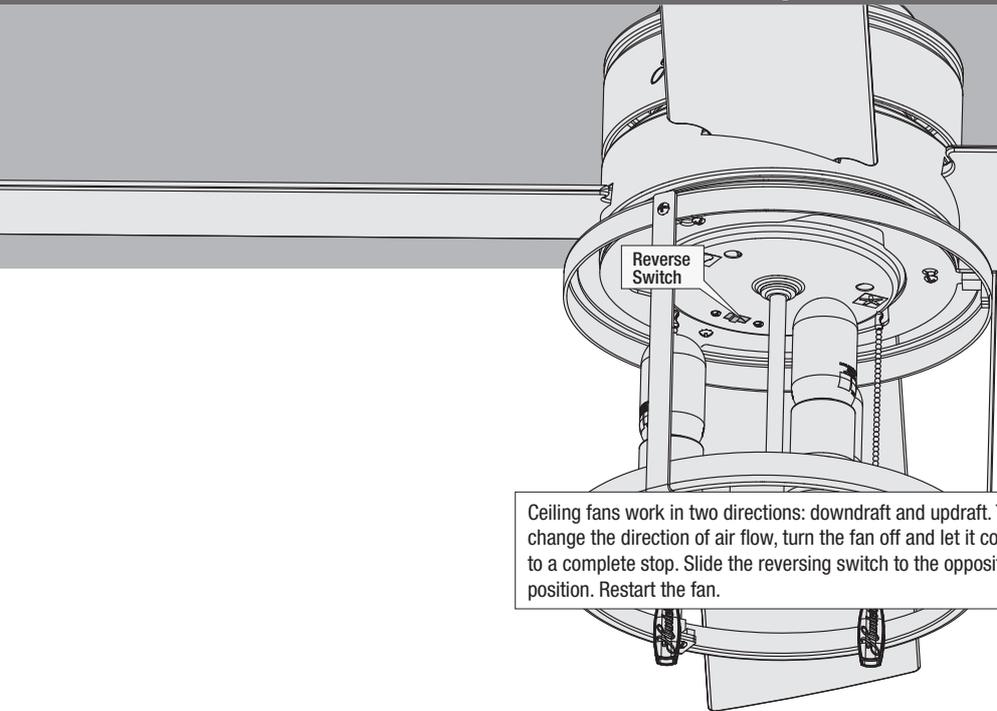
Ceiling fans work in two directions: downdraft and updraft. To change the direction of air flow, turn the fan off and let it come to a complete stop. Slide the reversing switch to the opposite position. Restart the fan.
