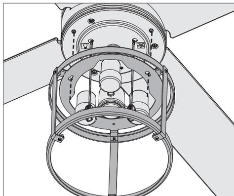
Lift cage assembly into place while passing pull chains through cage assembly as shown. Align the keyhole slots in the top of the cage assembly with the partially installed cage assembly screws. Wrap the keyhole slots around the screws and twist counterclockwise.
