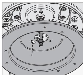
Feed the wire plug through the center hole of the upper switch housing. Align the keyhole slots in the upper switch housing with the two screws you just installed. Lift the upper switch housing so that the keyhole slots engage the two screws, and twist counterclockwise to lock the upper switch housing into place.
