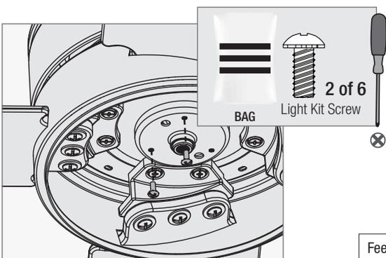
Partially install two light kit screws, found in the ≡ hardware bag, halfway into the motor housing as shown. It does not matter which two screw holes you choose.
