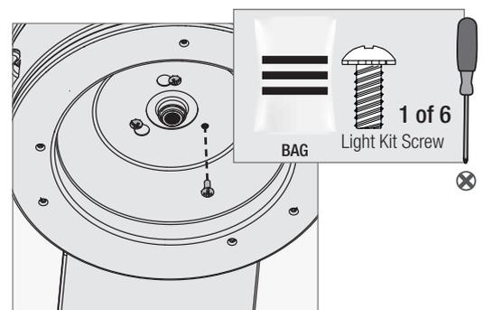
Insert the third screw, found in the ≡ hardware bag, in place and firmly tighten all the three screws.
