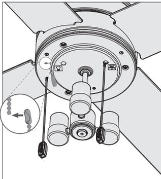
Remove and discard the plastic connectors from the ends of the short pull chain. Attach the pull chain pendants to the light and fan pull chains.
