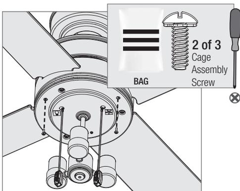
Partially install two cage assembly screws, found in the hardware bag, halfway into the light kit as shown. It does not matter which screw holes you choose.
