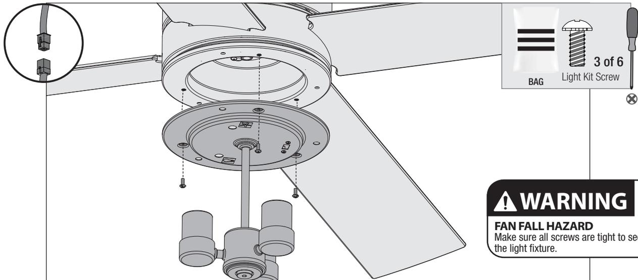
Connect the plug to the lower switch housing. Make sure to line up the colored markings on the connectors and that the connectors latch. Attach the lower switch housing to the upper switch housing using three light kit screws found in the hardware bag.
