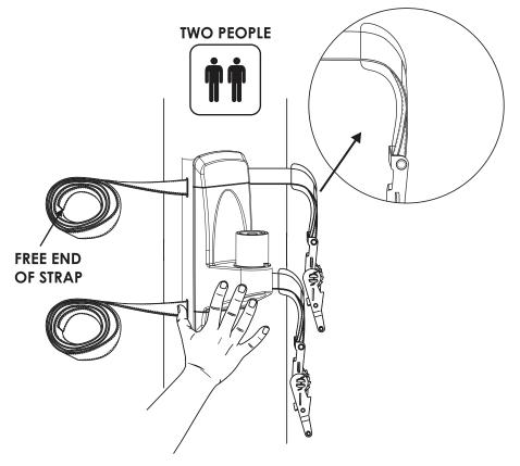
Hold column mounting bracket to the column where you would like to mount the monitor
