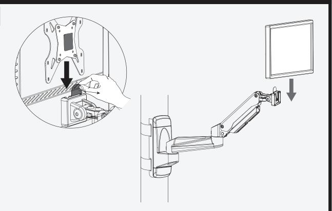
Lift the VESA plate along with monitor and put it on head slot.
