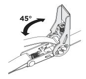
4b. Crank the handle to tighten the strap until it feels taut and secure.
