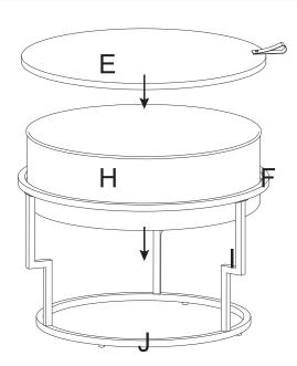
Place (H) into the frame formed by (F), (I), and (J), and support it with the metal plates on (F). Then place (E) into (H).
