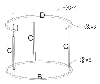
Insert (2) through the hole in (C) and tighten into (B). Insert (3) through D and tighten into (C). Screw (4) into the small hole in (D).
