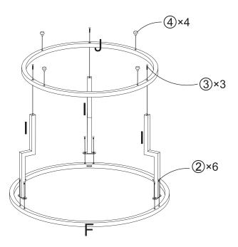
Insert (2) through the hole in (I) and tighten into (F). Insert (3) through the hole in (J) and tighten into (I). Screw (4) into the small hole in (J).
