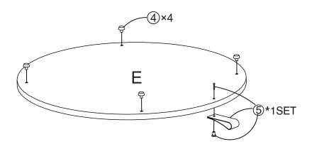
Insert the screw from (5) through (E) and the handle, and tighten into threaded rod.
