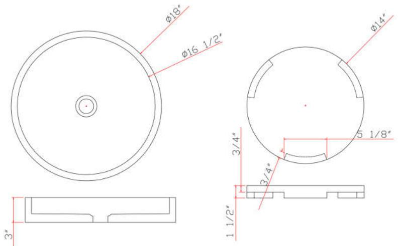
Dimensions of fixture are nominal and may vary within the range of tolerances established by ASME Standard A112.19.2. Dimensions and specifications subject to change without notice.
