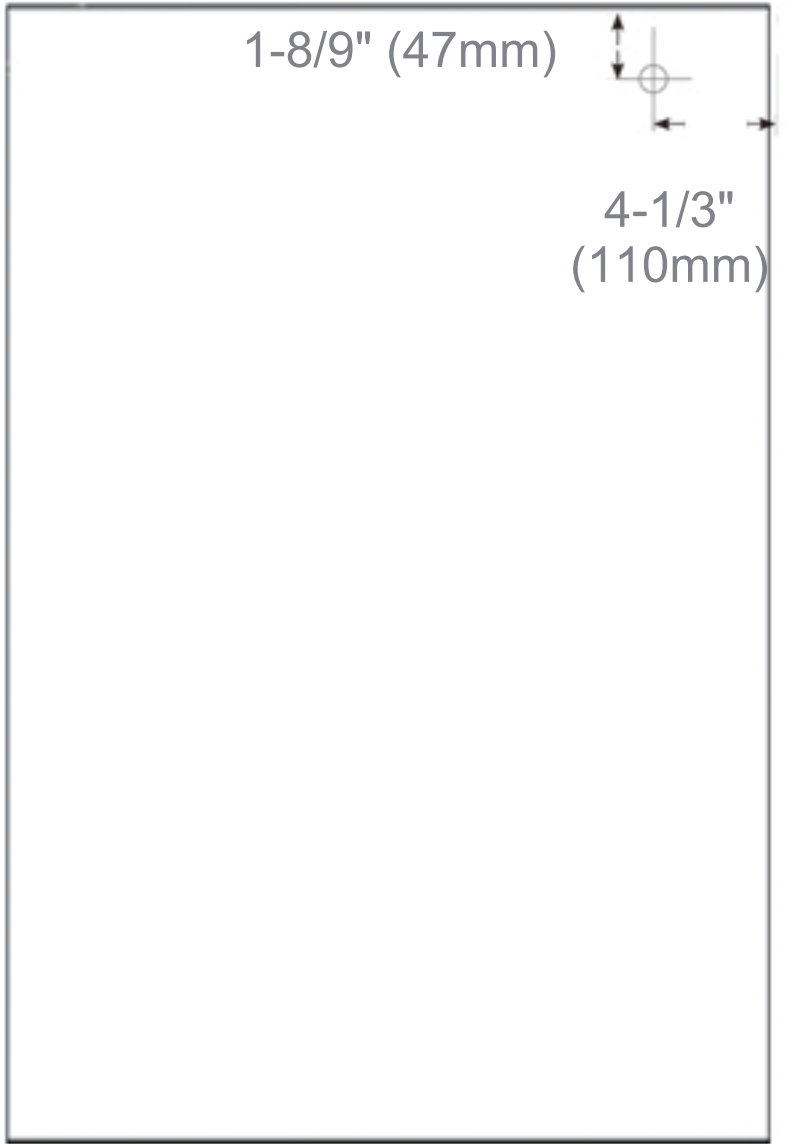
Back of Cabinet - Wire Access Location
