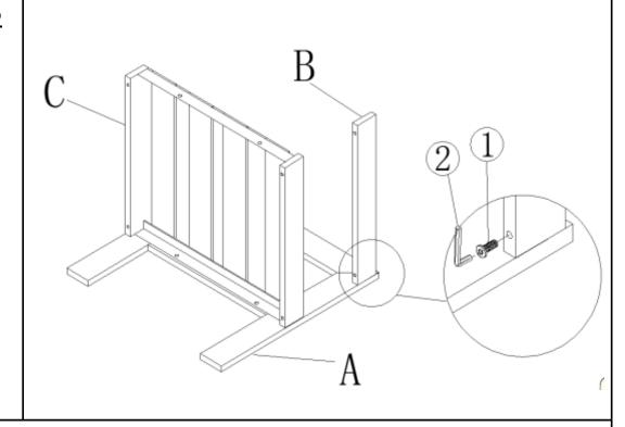
Attach the Back Support Bar(B) to the Side Panel(A) using Bolt(1) with Allen Key(2). **Do not fully tigthen Bolts.**
