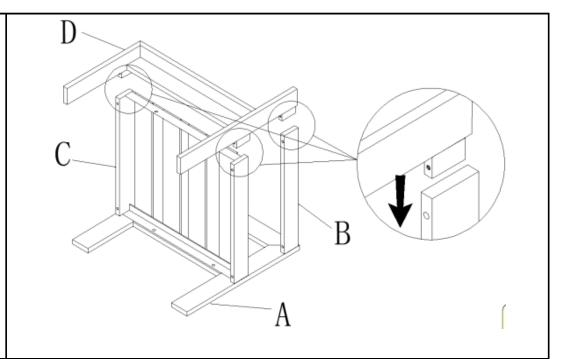
Insert the Leg Support Bar(D) into the Back Support Bar(B) and Seat Panel(C) as shown above.
