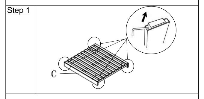
Open the carton and place all the parts onto a clean, non-marring surface. Remove the plastic plugs (prevent the alum tube was scratched) in the four ends of the Seat Board (C) using Allen Key(2) as shown above.
