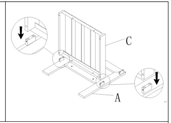
Place the Side Panel(A) with its inside facing up. Insert the Seat Panel(C) into the Side Panel(A).
