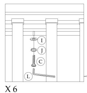
Check that the frame is central by adjusting the alignment of the frame and brackets before fully tightening all bolts. The metal frame should not contact the faux leather at any point.
