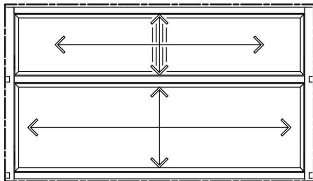
Insert the drawer into the main body, then adjust the drawer front panel left or right and up or down, until the drawer gaps look proportional.
