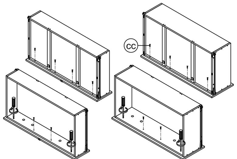
Pull the drawer open slowly and tighten the upper screws. Make sure the front panel does not move and lock the drawer front panel into position using Wood Screws (cc).
