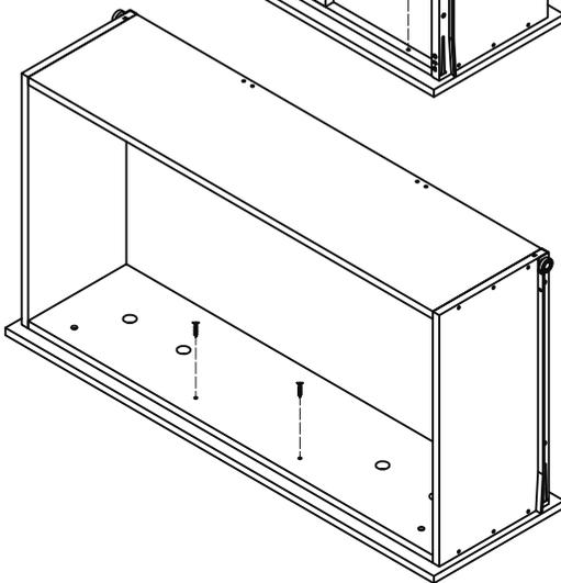
Pull out drawer slowly. Lock the drawer front panel into position using Wood Screws (cc).
