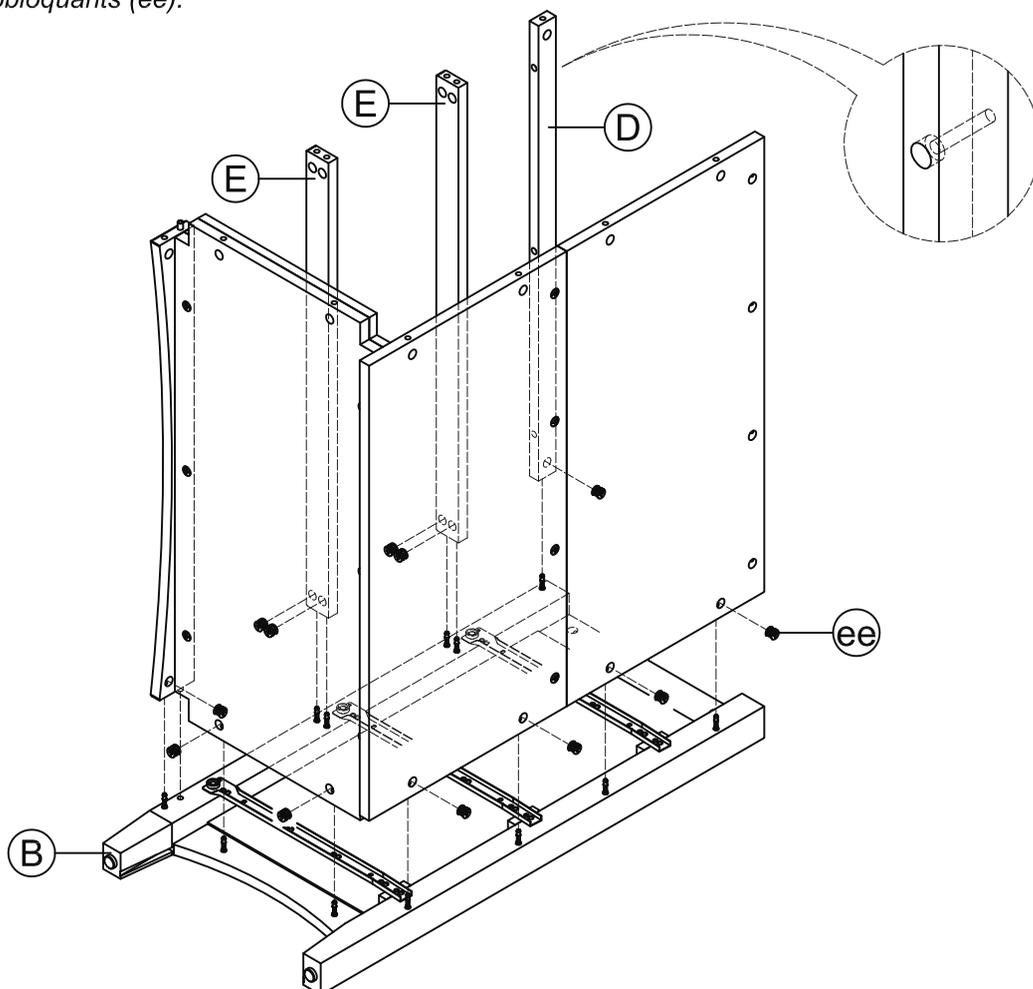
**5** Attach Right Assembly (C) to unit using Camlocks (ee).
