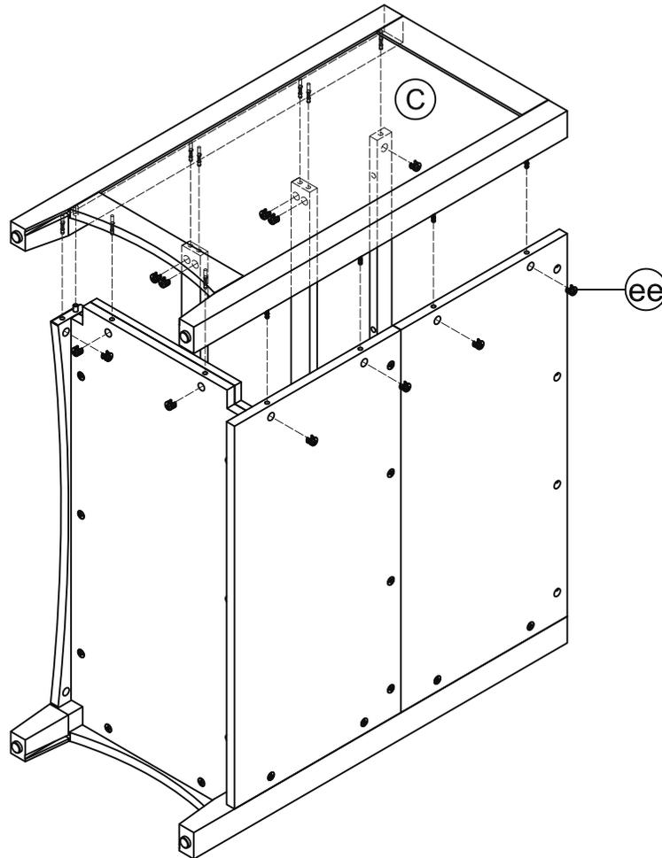
**6** Attach Top Panel (A) to unit using Camlocks (ee) and Wood Screws (aa).
