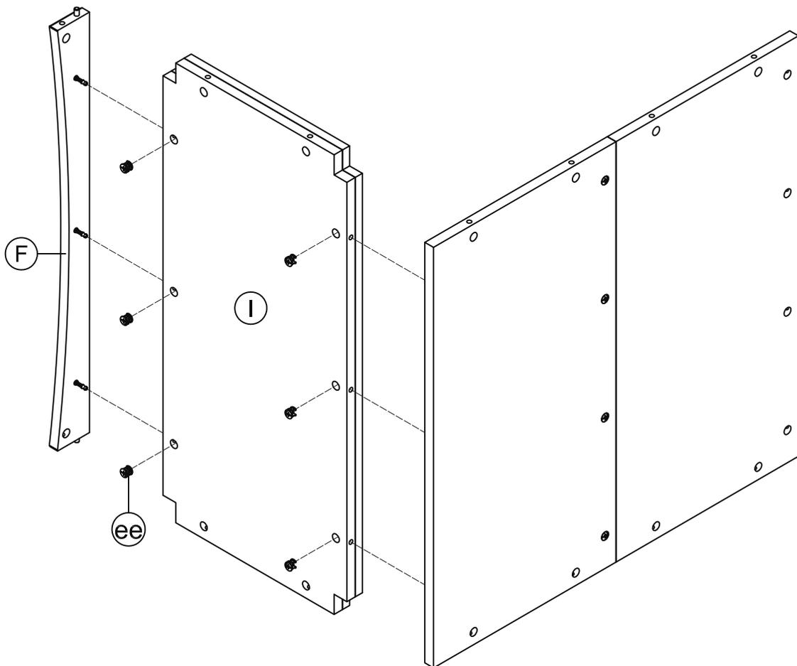
**4** Attach unit, Upper & Middle Frame (D) & (E) to Left Assembly (B) using Camlocks (ee).
