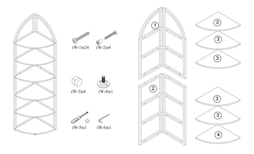
**Notes:** Don't tighten screws completely at first, just in case parts were assembled wrong and need disassembled. Tighten screws at last when all parts are put together.
