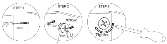
Push the KD cam all the way into the hole before tightening.
