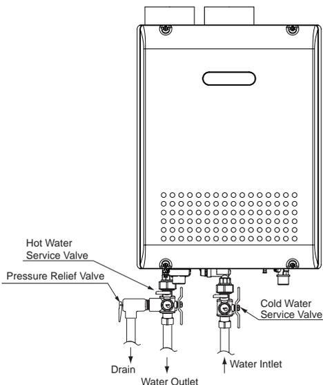
\* Isolation valves may be purchased as an accessory from Noritz. They allow for full diagnostic testing and easy flushing of the system.
