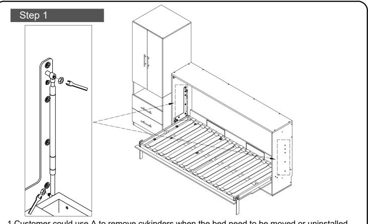
1.Customer could use A to remove cykinders when the bed need to be moved or uninstalled 2.Loosen the screwof the cykinders
