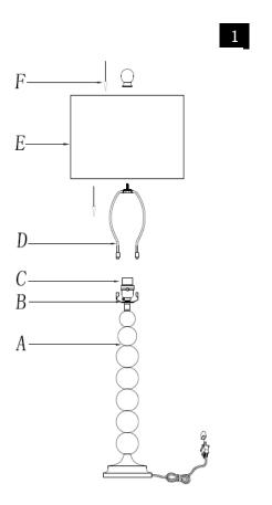
Step 1 Unpack all parts from cartons carefully Insert the Harp (D) into the Saddle (B). Put the shade(E) on the Harp(D), then tighten the Finial (F)into the Harp (D)
