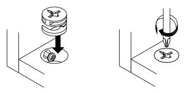
Turn cam lock clockwise to tighten.
