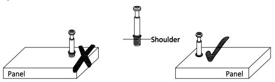
Tighten quickfit until shoulder is flush with panel. Do not overtighten or undertighten.
