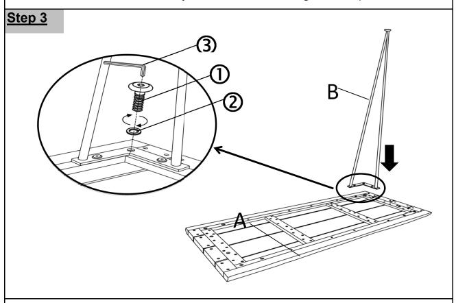
Insert one of legs (B) into the table top (A), put the flat washer (②) and bolt (①) as above picture.
