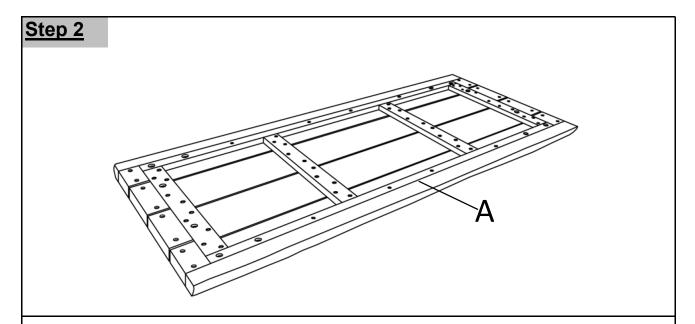
With the assistance of an adult, lay the Table top (A) facedown onto a clean, flat surface to avoid any scratches or damage to the product.
