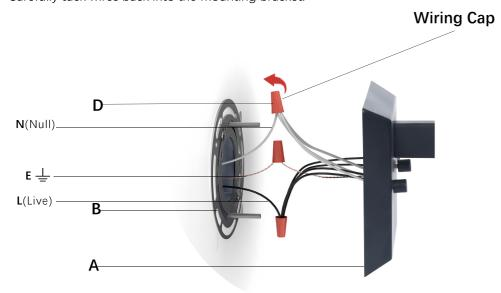
**STEP 5**Place the fixture(A) over the mounting bracket(B), use the nut(F) to attach them.
