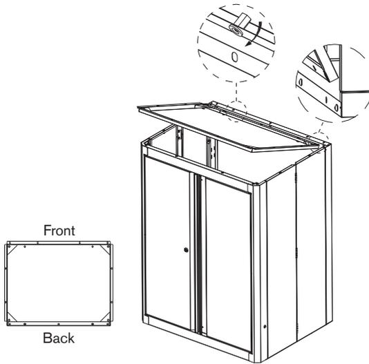
Attach the bottom panel using eleven M6 x 16 hex socket head screws.
