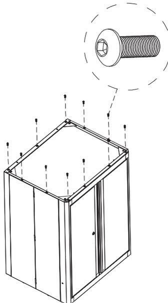
Attach the top panel to the cabinet using eight M6 x 16 hex socket head screws.
