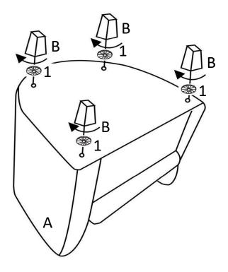
Place Chair (A) on its back on a flat smooth surface. Attach Feet (B) and Washers (1) to Chair (A).
