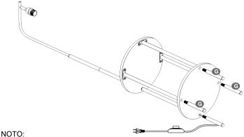
Pull out any excess power cord through the Tube-G1, Screw the Tube(G&G1) clockwise onto the Tube-F until tight.
