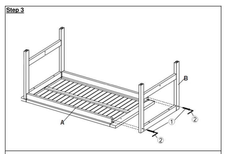
Repeat the same process to affix 2nd Leg Panel (B) to Table Top (A) by using Screws (1) and Allen Key (2) LOOSELY TIGHTEN THE SCREWS, up to 50%.
