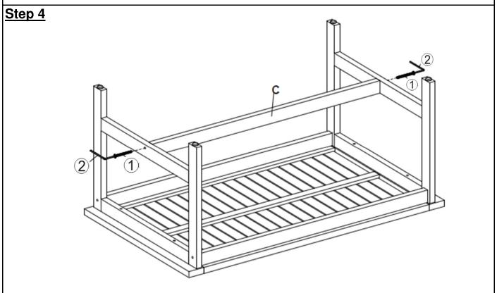
Affix Support Bar (C) to Leg Panels (B) by using Screws (1) and Allen Key (2). You may need to push the Leg Panels (B), outwards, slightly to attach the legs. **LOOSELY TIGHTEN THE SCREWS, up to 80%.**
