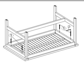
Use Screws (1) and Allen Key (2) to attach Table Top (A) and Leg Panels (B).
