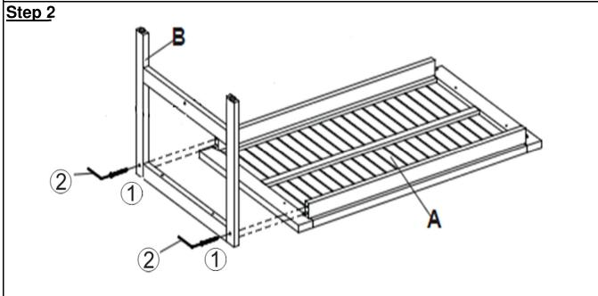
Position Table Top (A) and Leg Panel (B) as shown in picture above. Then affix 1st Leg Panel (B) to Table Top (A) by using Screws (1) and Allen Key (2) **LOSELY TIGHTEN THE SCREWS, up to 50%.**
