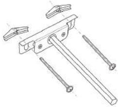
The open part of the wings should be facing the head of the bolt.
