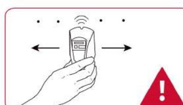
03 Determine if there are studs behind the wall where you want to mount the bracket
