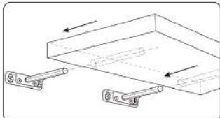
Insert the shelf onto the installed brackets.
