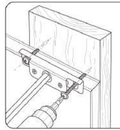
Mount the screws (included) with bracket into the wall where there is a stud
