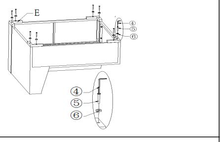
Attach the Foot(E) to the Chair using Bolts(⑤) and Washer Rings(⑥) with Allen Key(④).
