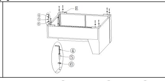
Attach the Foot(E) to the Chair using Bolts(⑤) and Washer Rings(⑥) with Allen Key(④).
