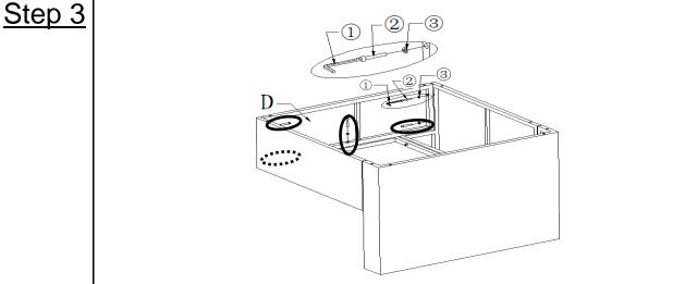
Attach Side Plate(D) between the Back(I) and Seat(J) using Bolt(2) and Washer(3) with Allen Key(1) as shown above.
