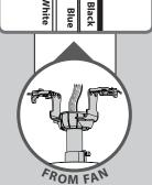
Turn the splices upward and push them carefully back through the hanger bracket into the outlet box. Spread the wires apart, with the grounded wires on one side of the outlet box and the ungrounded wires on the other side of the outlet box.
