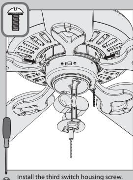
Tighten all three screws securely.
