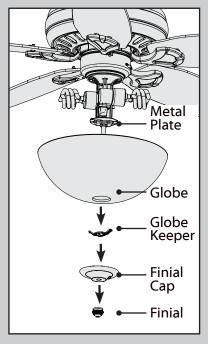
Changing the bulbs - unscrew the finial and remove it from the threaded rod. Remove the finial cap and unscrew the globe keeper while supporting the globe with your other hand. Carefully remove the globe. Unscrew bulbs and replace with bulbs of same type and wattage. Reinstall the globe assembly.
