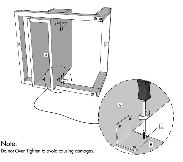
Attach E to Assembled Night Stand using a Philips Screwdriver as shown.
