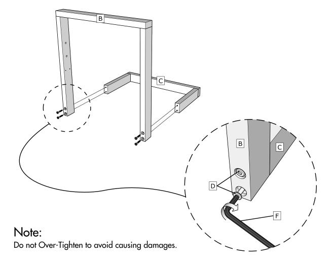
Attach  $\square$  to  $\square$  with  $\square$  using a Ball End Hex Key Wrench  $\square$  as shown.
