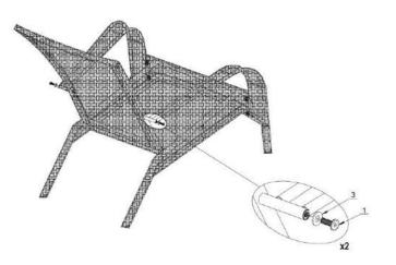
**Step 2:** Attach the Arms to the Seat Back with 2 - pcs. M6x20 Bolts and M6 Washers with the Allen Wrench.
