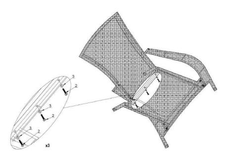
**Step 3**: Attach the Seat to the Seat Back with 3 – M6x40 Bolt and M6 washers with the Allen Wrench.
