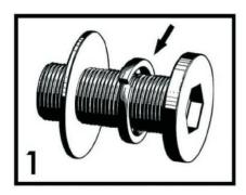
When lock or spring washer is used in an assembly, please make sure the lock or spring washer is placed between the larger flat washer and the head of the screw or bolt.
