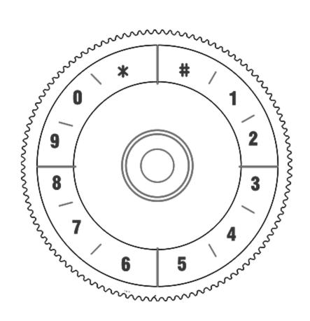
2. Enter any new 3-12 digits code, press the "#" button to confirm. The buzzer will sound once and the blue indicator light will be off. Password is set successfully.
